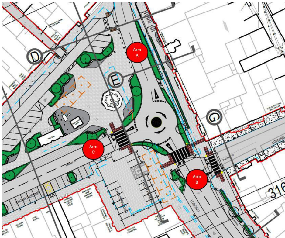
Figure 8.3: Proposed mini-roundabout modelling layout
